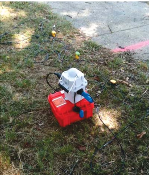
Example of a Seismic Monitoring System (Normally in place for a 20+ day period)
