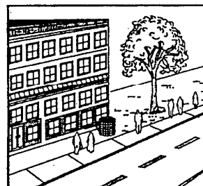
#19 Inappropriate front location for mechanical equipment
